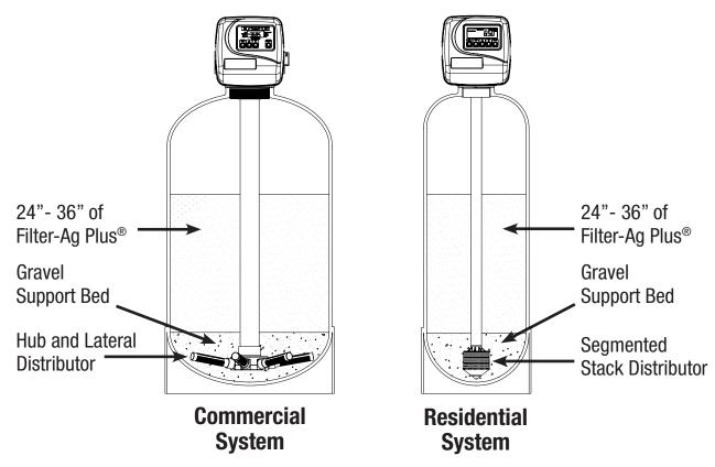
Before putting Filter-Ag Plus® filter into service follow these recommended instructions or contact the original equipment supplier
